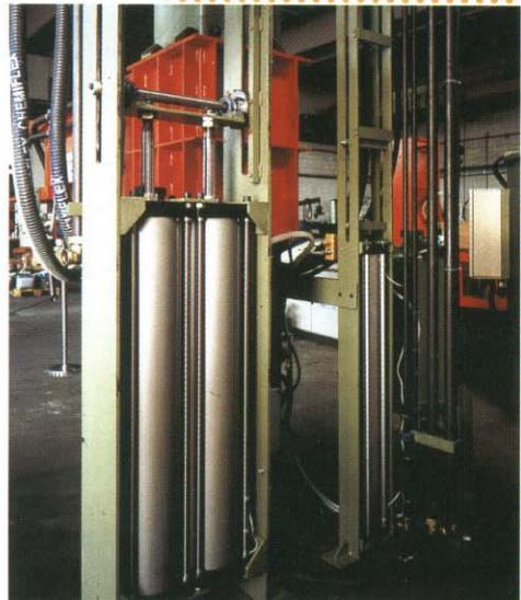
**1° phase:** preparation of resins (polyol + additives + blowing agent) for BB3 or water activator (water + additives) for BB4
